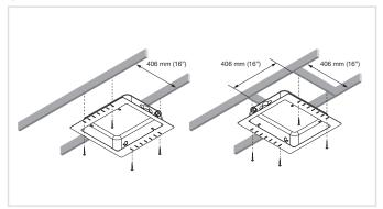
Install the back box onto the supporting beams in the wall or ceiling. The back box can be installed in both horizontal or vertical direction. Use the provided slots for mounting the back box to the supporting beams. Depending on the structural material the appropriate fasteners shall be used.
