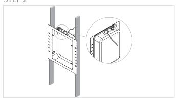
Assemble the cable gland through one of the provided knock-out holes in the back box, and provide the cable through it. Loop the cable through the bracket on top of the back-box, to avoid stress on the cable and contacts. Make sure the cable gland is well tightened to avoid any air-leakage through it.
