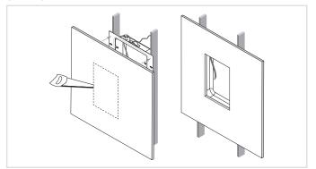
Finish the structure by placing finishing board (plasterboard, wood, ...) in front of it. Make the cut-out for the installed speaker according to the required dimensions. Afterwards, connect, insert and install the speaker into the provided opening.
